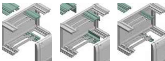
Bus, rear and snap profiles for the fitting of 19" components
